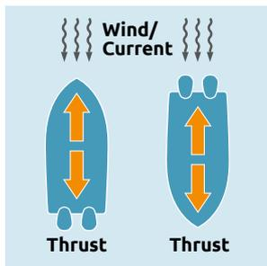
Keeps position. This mode uses minimal RPM to hold your position. Perfect for stationary fishing.
