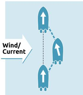
Holds the vessels course automatically adjusting for wind or current drift.
