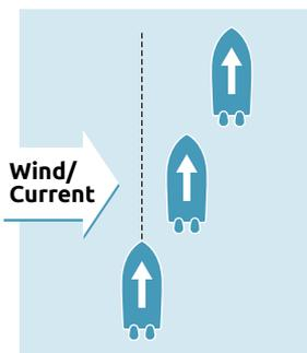
Holds the vessels compass setting. Applicable also to reverse shift for enhanced back trolling.
