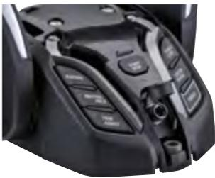
The easily accessible port helps Yamaha dealers connect YDIS for system compatibility scan, diagnosis and updating software.
