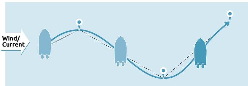
Keep the heading and drift to trace the waypoint (s) which you set from MFD - like following same depth contour or keeping distance from shore. You can enter this mode to push DRIFTPOINT button when MFD navigation route is set.
