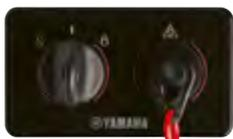
1 - SINGLE ENGINE KEY SWITCH WITH LANYARD
