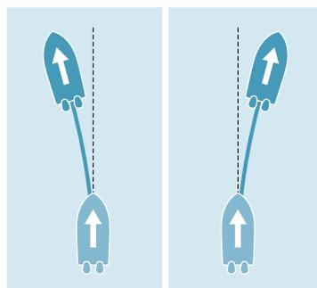
Press this button to change the set heading of your boat at Heading/ Course Hold modes. Short press : 1 degree increment. Long press : 5 degrees increment. Hold the button down for further steering.
