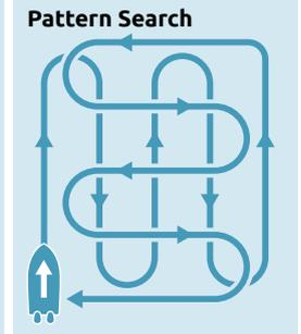
Pre-selected patterns that are adjustable - Spiral and Zig-zag - useful to find signs of fish at a target spot.
