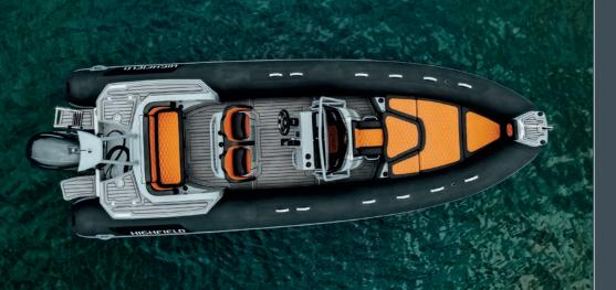
The Sport 700 is a boat at home when the weather gets up. The 26 degree deadrise hull eats the chop and keeps you and your family dry and secure in all conditions. Self draining decks and a 140 litre fuel tank allow you to maximise your time afloat.
